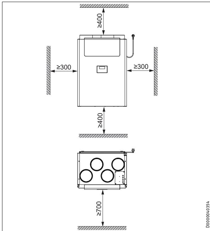
Installation drawing with silencer attachment
